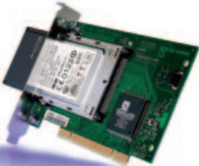
ORiNOCO wireless technology is the freedom to build a wireless LAN in your home, small office or enterprise Anytime. Anywhere. And any way you want. The ORiNOCO 11b PCI Adapter simply sits in a free PCI slot. Once locked on the board, the 11b PCI Adapter forms a Wireless Network Interface Card (NIC). The 11b PCI Adapter extends wireless LAN access to desktop PCs and is compatible with all IEEE 802.11b compliant wireless LAN systems.
